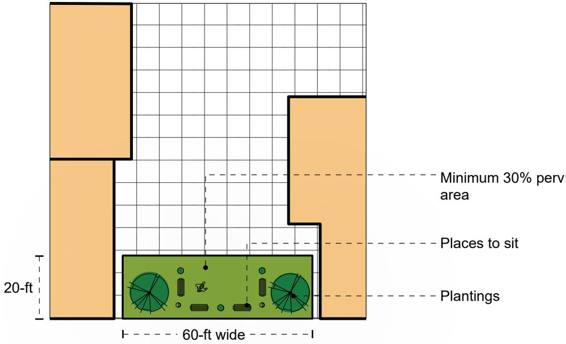
Figure 15: Pedestrian street concept diagram
