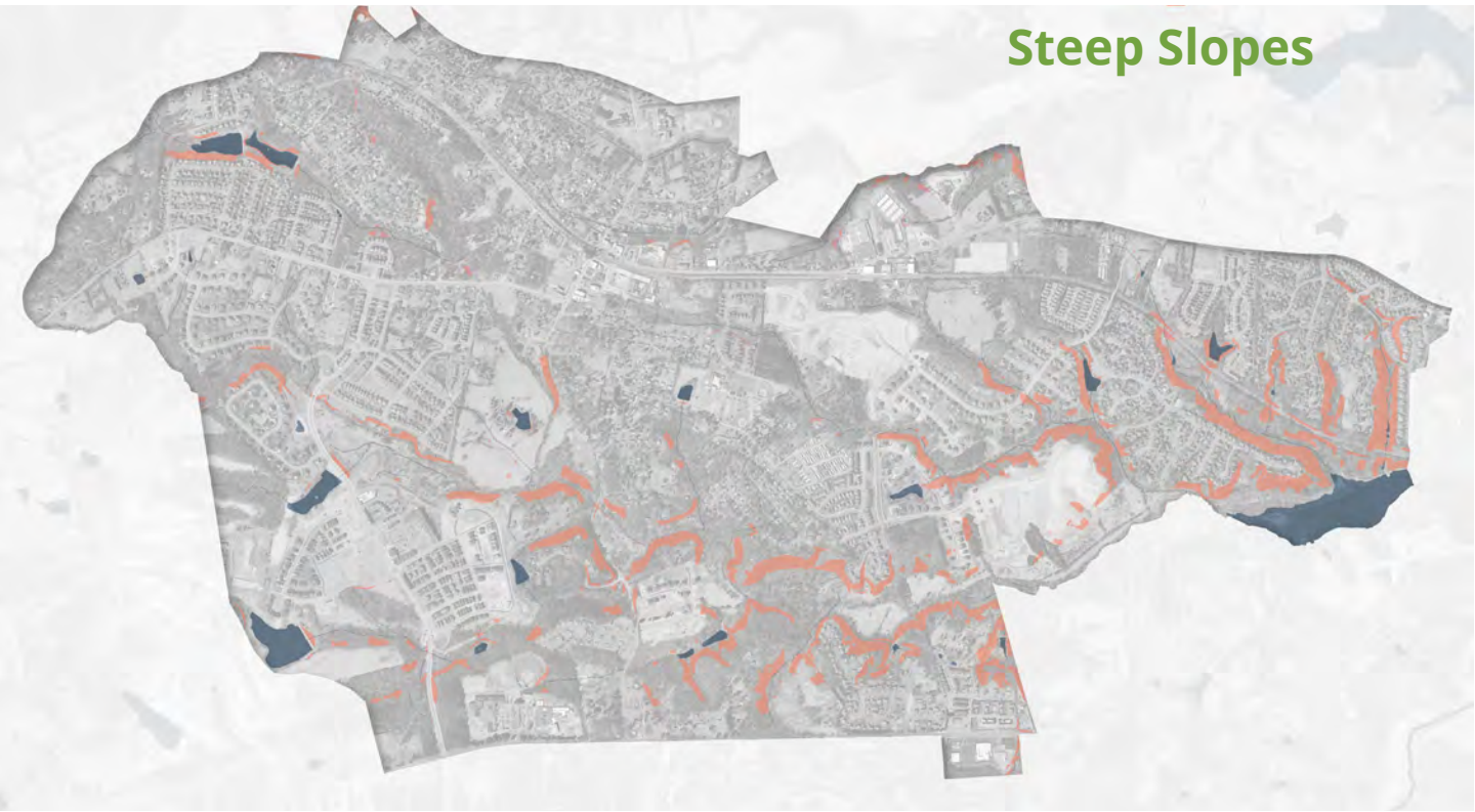
The map above shows areas within preserved steep slopes in light pink. Steep slopes are areas of incline with a 25 percent grade or greater (grade refers to the angle of the incline, where horizontal or flat equals zero). Steep slopes are regulated through a steep slopes overlay district in the Albemarle County Zoning Ordinance.
