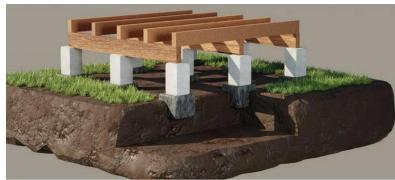
To minimize below grade disturbance we are also proposing **shallow** pier footings as opposed to a spread footing and continuous foundation wall.
