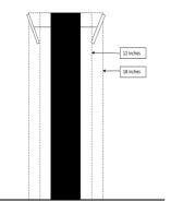
This special exception request is to increase the distance of the farthest point of the back of the proposed antenna from 18 inches to 30 inches from the facility. The proposed antenna would comply with all other ordinance requirements, including the size limit of 1,400 square inches.
