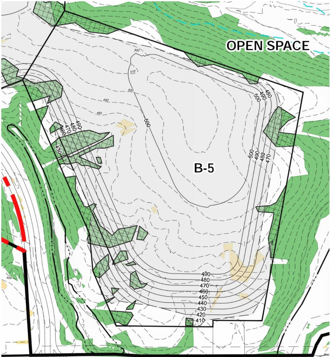
The project proposes to disturb the critical slopes located within the boundaries of area B-5, as shown above. These areas are noted in both light yellow and green with crosshatching. These critical slopes are located in multiple groupings ranging in size from 404 square feet to 35,500 square feet (0.8 acres). The procedure and criteria for evaluation of the special exception are contained in County Code § 18-4.2.5.
