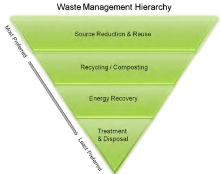
The 'Waste Management Hierarchy'. The management strategies are ranked in order of most to least environmentally preferred.
