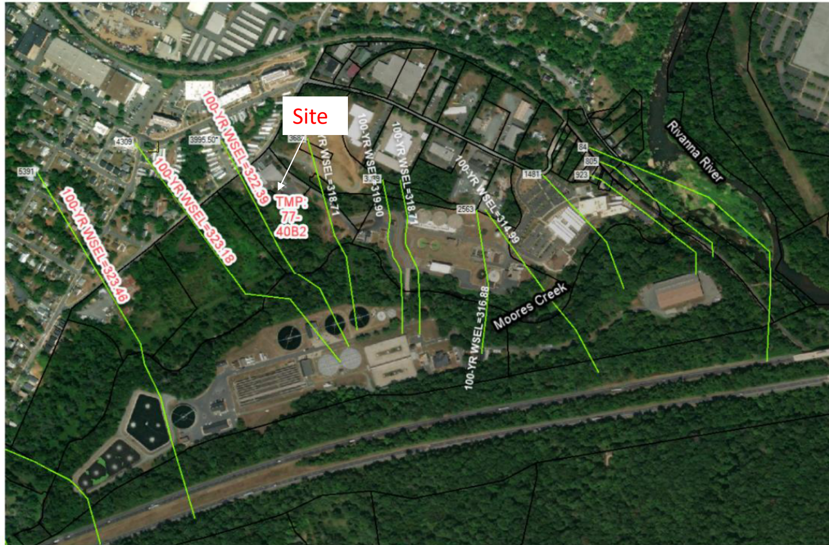
Figure 6: Resulting 100-YR WSEL With Addition of Ineffective Flow Area in Cross Section 3995.50
