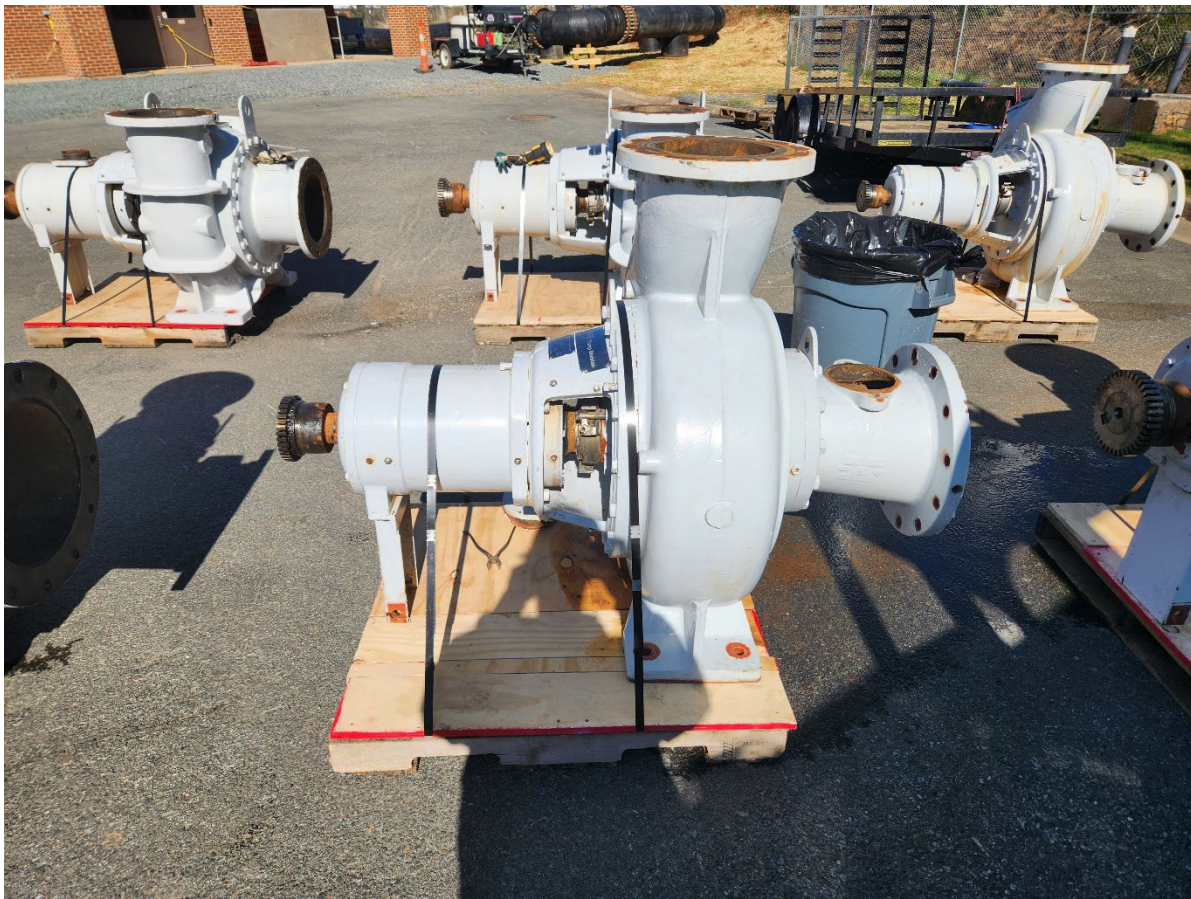
Pumps removed from pump station.
